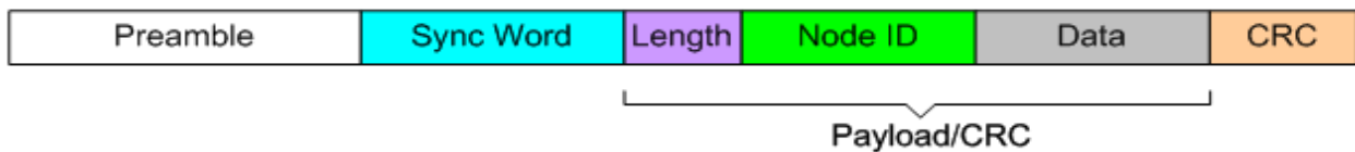
Figure 15. Variable Packet Format, Node ID Exists, Node ID is after Length Byte
